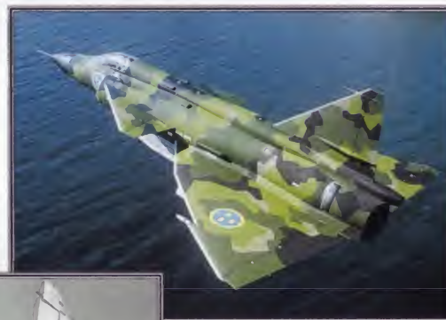
◀ Short landing run Slots in the rear fuselage are connected to the nosewheel and open upon landing to direct the engine thrust forwards.
